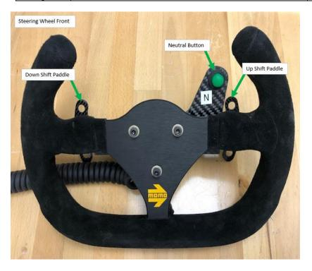
To select first gear with the car in neutral. Depress clutch. Press Neutral button and 1 click on the upshift paddle. Make sure '1' is displayed on the dash.
